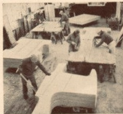
FLOOR BOARDS BY THE BUNCH for GMC buses are turned out year round by workmen using special jigs and cutting tools developed by Emmanuel Pasquier. Plant has doubled in size in past five years, present plans call for plant to soon double in size again.
