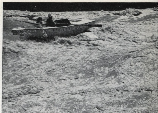
SUPER-Harbord was used as bottoms, sides, decks, bulkheads, seats, cowling, air chambers, etc. of three cataract type boats used by Nevills 1938 Colorado River Expedition.
